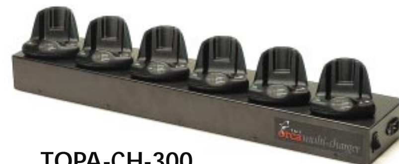
TOPA-CH-300 • Multi-Charger (six independent fast chargers) • Battery Conditioning • Conditioning/Analysing
