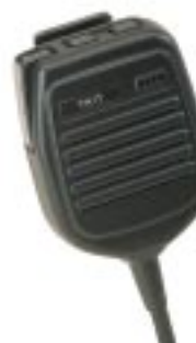
TOPA-AA-002 • -30C / +60C Rainproof • 2 Programmable Function Buttons • Top Connector
