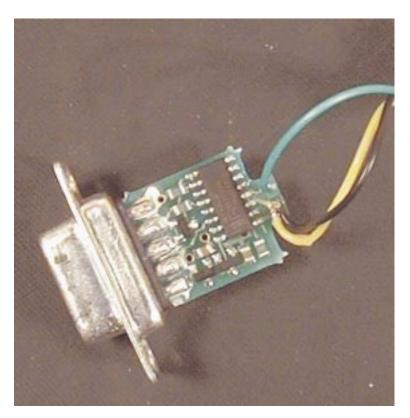
Apply low temperature hot melt glue (eg RS part no 692-441) to the cable entry/clamp area. This glue prevents fretting of the cable & premature breakage.
