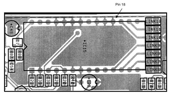
Figure 6 T800-30-0002 Location of Pin 18 - Top Side
