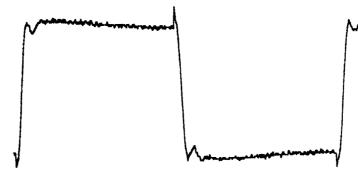
Figure 7 100Hz VCO Control Line Waveform
