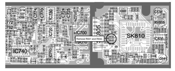
Figure 3 T800 Series II Microcontroller Compartment - Top Side
