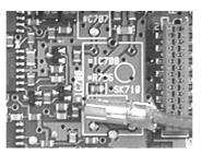
Figure 1 Location Of Socket And SMD Resistor
