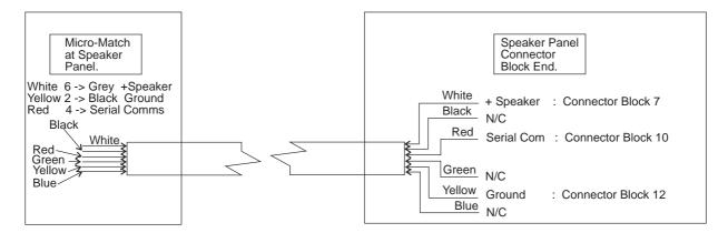
Figure 1 Speaker And Programming Port Wiring Details
