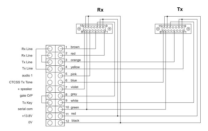
Figure 3 T800-23-0000 Loom Wiring Details
