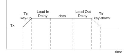
When data is detected at the radio's input buffer, the following occurs:
