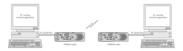
When in Command mode, commands and response messages are passed between the PC and the radio using the CCDI protocol. CCDI commands can also be used to obtain GPS data and NMEA messages from the radio. Refer to "QUERY" and "SEND\_ADAPTABLE\_SDM". The baud rate is set to 1200, 2400, 4800, 9600, 14400, 19200, 28800 or 115200 (TM8200 only) baud, using the programming application.
