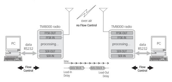
Transparent mode data is packetised into data blocks before it is sent overair. The start and stop bits are removed and a header is sent at the start of each data block.
