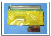
If the LCD assembly is to be fitted to a <u>Tait Orca Excel or Eclipse</u> then you need to place the foam pad (IPN 369-02060-00) just to the right of the black bulge on the back of the LCD module. The resulting LCD assembly with foam pad fitted is shown below.
