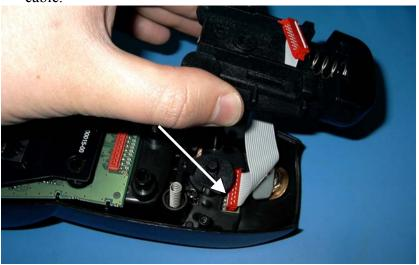
8) Remove the two springs, the peg moulding and quarter turn moulding.
