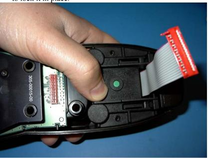
13) Test the locking mechanism works.
