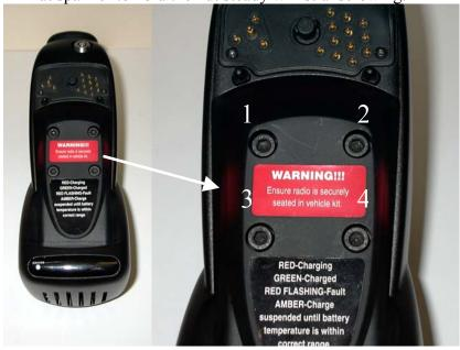
3) Using the end of a flat head screwdriver. Apply pressure to one of the retaining clips. With the other hand gently pull the back cover away. Repeat process for other retaining clip. Then lift the back cover upward to remove.
