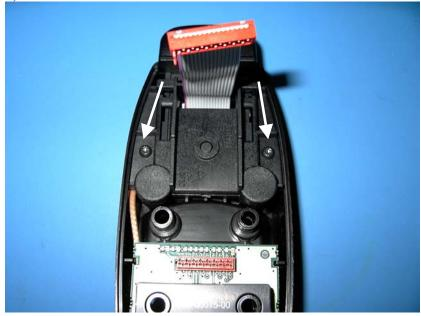
6) Gently remove the top portion of the trigger assembly by lifting it upward.
