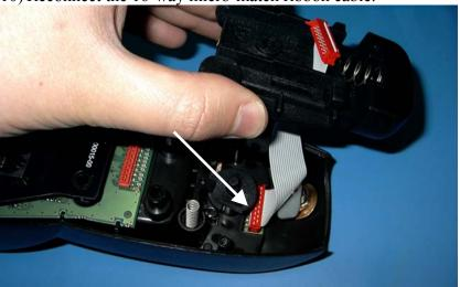
11) Hold down on the top housing and spring whilst refitting the trigger assembly cover.
