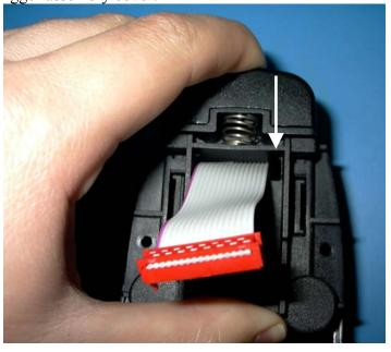
12) Push firmly down on the rear of the trigger assembly cover to lock it in place.
