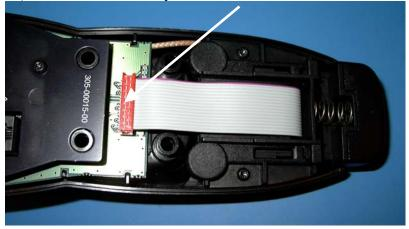
16) Refit the back cover. Line up the end nearest the top trigger assembly, and then push the other end downward until the retaining clips click into place.
