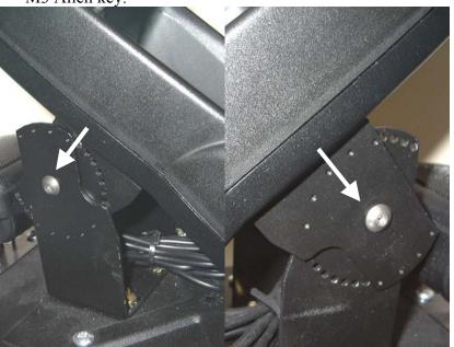
2) Next use an M4 Allen key to remove the four screws that hold the bracket to the vehicle kit. If necessary, use an M5 nut spanner to hold the nut steady whilst unscrewing.
