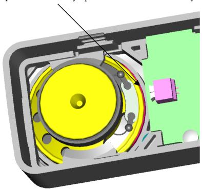
Fit label into groove with adhesive side facing towards Keypad. Position it so that it label rests in the bottom of the groove. Use a blunt instrument such as an iceblock stick to press the adhesive onto the curved face of the outer speaker ring. The label will sit approx 1.5 to 2mm above the outer speaker ring.
