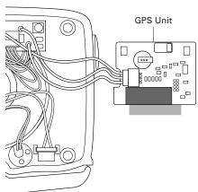
**Note:** Remove cables connected to the GPS unit, if needed.
