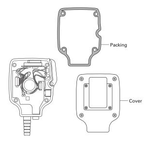
3. Remove the GPS unit installed in the upper part of the microphone.
