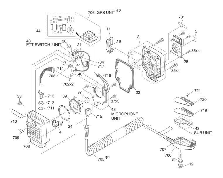
\$1: In order to maintain the waterproofing performance, the cord ASSY with plug cannot be replaced. \$2: The GPS unit cannot be replaced.
