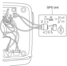
**Note**: Remove cables connected to the GPS unit, if needed.
