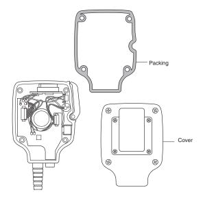
Remove the GPS unit installed in the upper part of the microphone.
