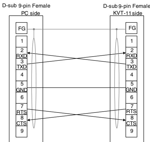
**Fig. 2 Cable assignments**
