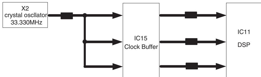
Fig. 5 Clock circuit
