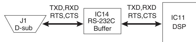
Fig. 3 Serial interface circuit
