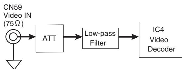
Fig. 2 Video decoder circuit
