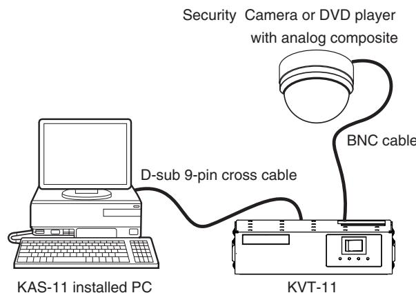
**Fig.1 Connection diagram**
