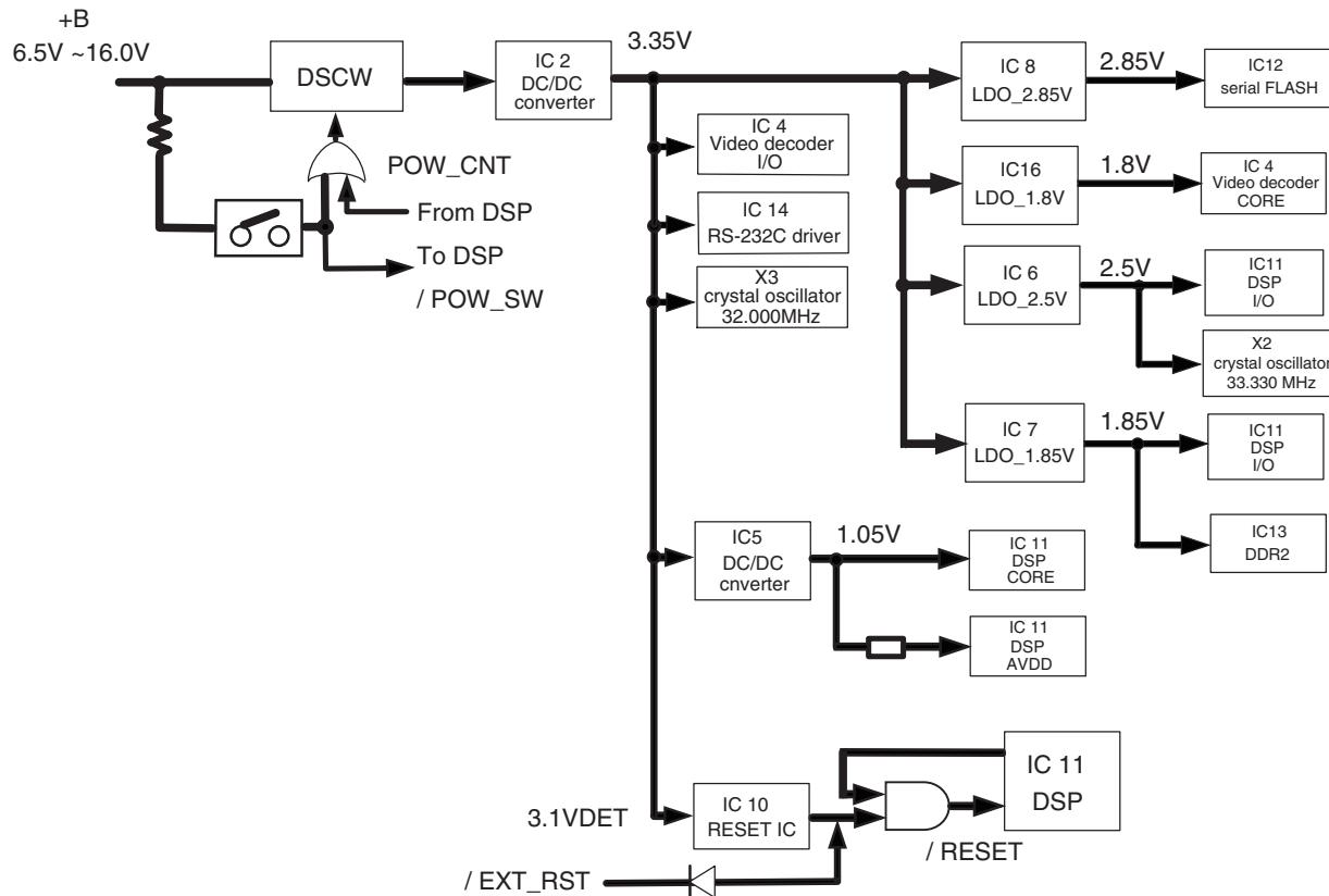
Fig. 4 Power supply circuit
