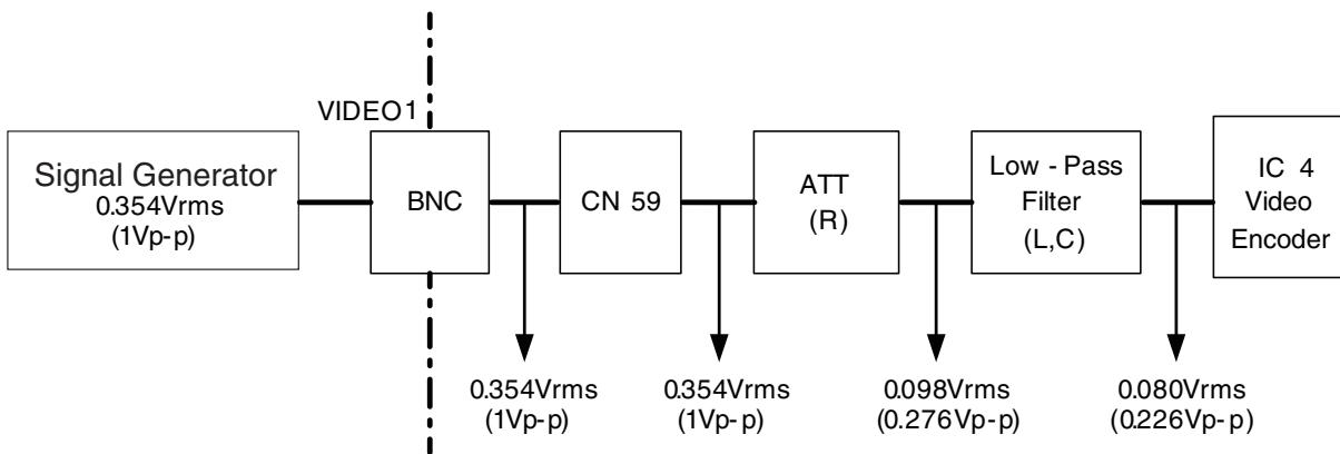
All voltage values are measured by using an oscilloscope when 0.354Vrms(1.0Vp-p) is applied to the BNC terminal.
