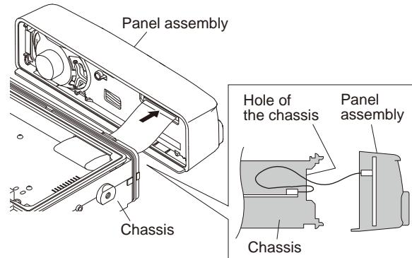
3. Fit the panel assembly into the two tabs of the chassis top side first.
