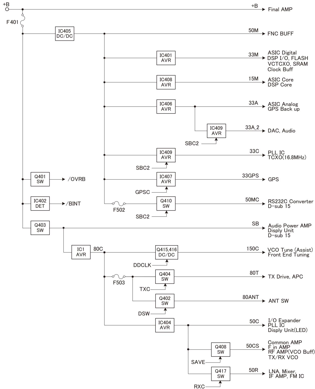
Fig. 16 Power supply circuit
