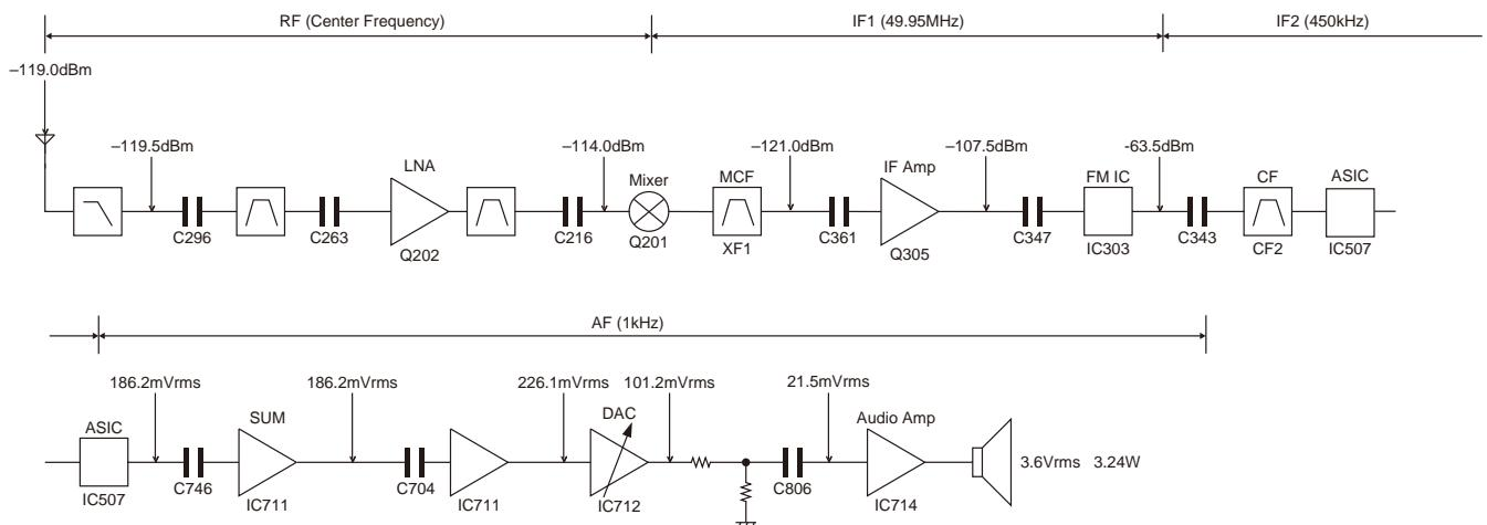
To make measurements in the AF section, connect the AC level meter. (ANT input: -53dB, 1kHz FM, 3kHz DEV (Wide))
