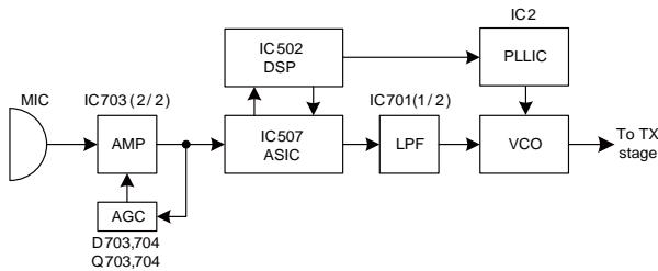
Fig. 4 Transmitter System
