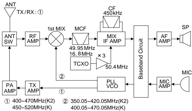
**Fig.1 Frequency configuration**
