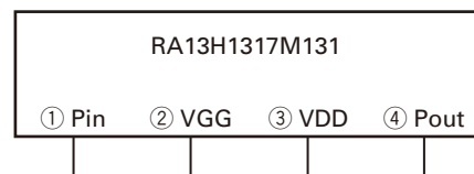
Fig. 9 Transmitter power module
