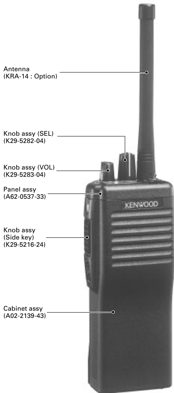
Photo is TK-290 K type. Does not come with antenna. Antenna is available as an option.
