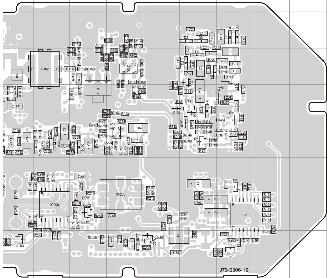
TX-RX UNIT (X57-8100-23) Foil side view (J79-0306-19)
