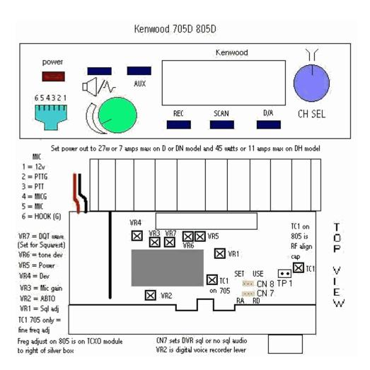
VR4=max deviation set, VR3=Mic sensitivity set, VR7=dig waveform bal (set for squarest digital waveform as seen at output frequency on service monitor), VR6=PL tone level (500 to 750 ~), VR5=power out (set to 27W) right side of silver VCO box VR1=preset squelch level, VR2=ABTO (this is the level control when using the digital audio recording option board).
