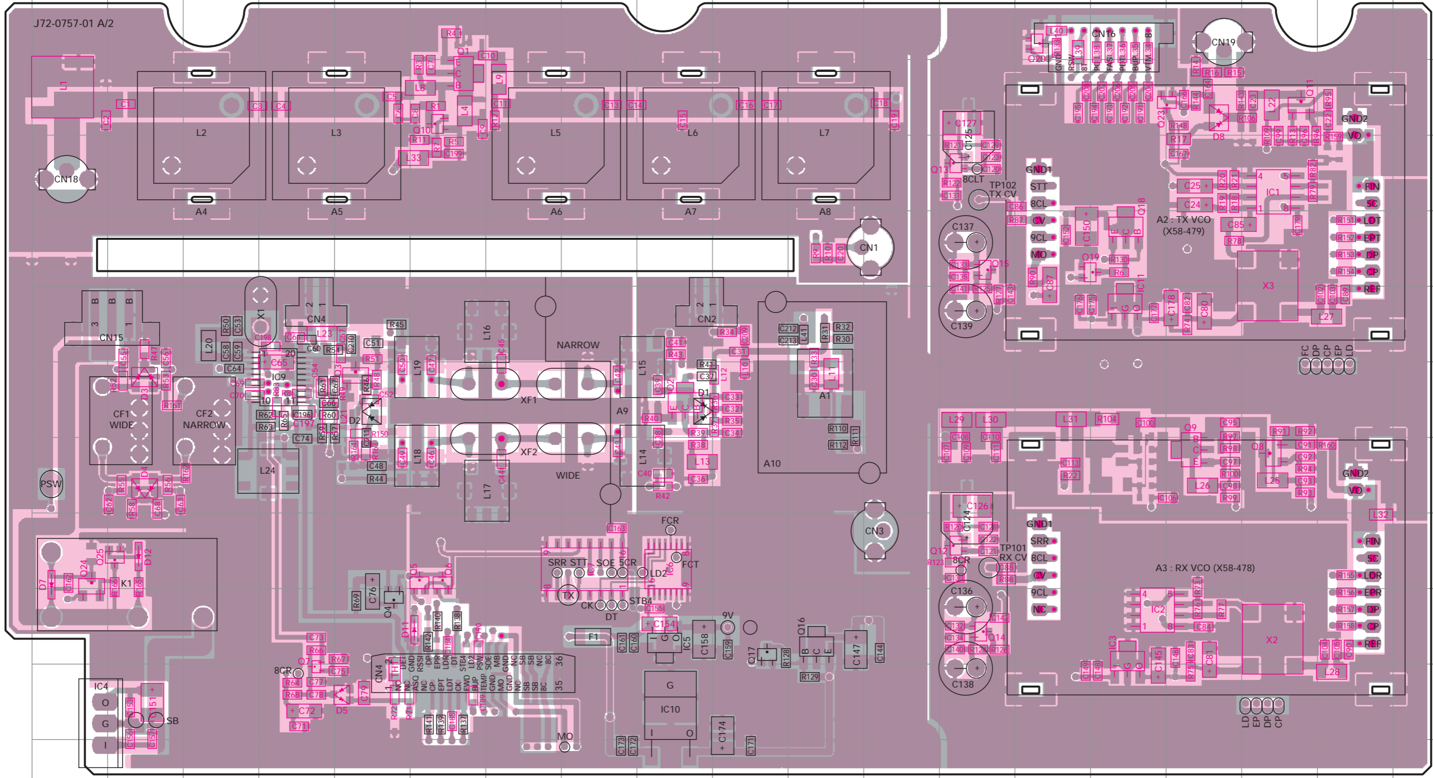
TX-RX UNIT (X57-6260-XX) (A/2) -10 : K,E -11 : K2 Component side view + Foil side
