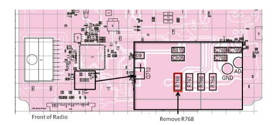
**Caution:** This modification requires soldering equipment rated for CMOS type circuits. It also requires familiarity with surface mount soldering techniques. If you do not have the proper equipment or knowledge, do not attempt this modification yourself. Seek qualified assistance.
