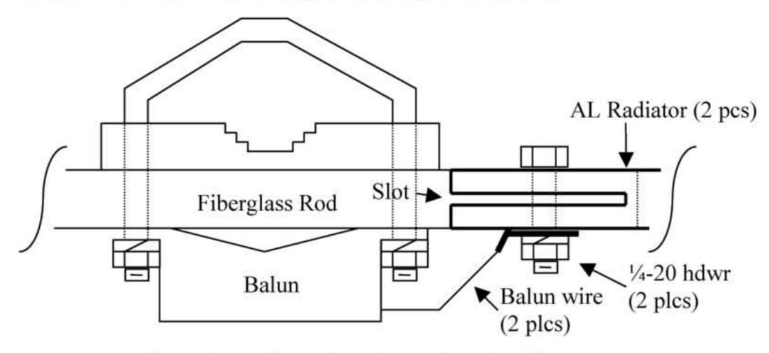
Figure 3: Radiator Tube Assembly - Top View
