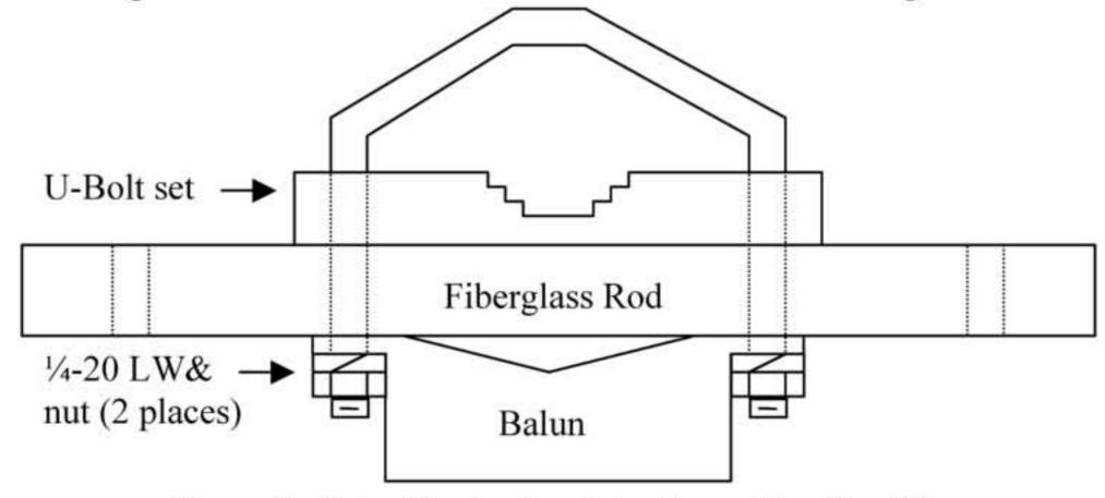
Figure 2: Balun/Center Insulator Assembly – Top View
