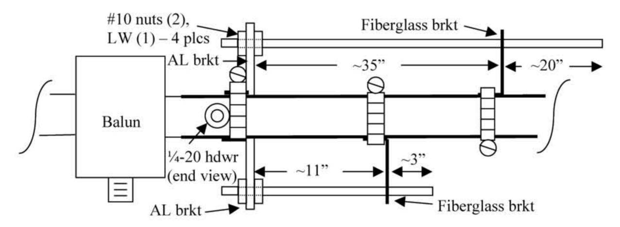
Figure 4: 6 and 2-meter stub assembly and mounting
