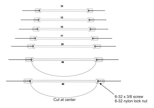
Install the 30-40 meter insulators by aligning them with the 10-20 meter insulators. Pull the wire and tension each side equally. Allow the wire to sag enough so that the tension is very small. Allow excess wire to sag under the insulator. Loop the wire around the screw and tighten the nut. Cut the excess wire in the center of the sag. The excess wire that hangs down will be used to tune the antenna.
