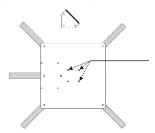
Remove three of the screws from middle of the top plate. It doesn't matter which 3 of the 4 you choose. The support arms shouldn't move with the element wires holding them in place.
