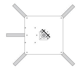
Install u-bolt and support tube. The tube should rest on top of the plate. Tighten the u-bolt snug but do not crush the tube.
