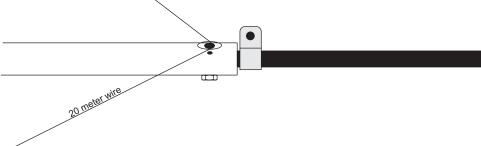
Take the support rope supplied and cut it into 4 equal sections. Use one section for each element arm. Double loop one end around the spacer inside the clamp. Leave about 3 inches excess and use the cable ties to secure it back to itself as shown. Use 3 ties and pull them tight. Repeat for the other arms.
