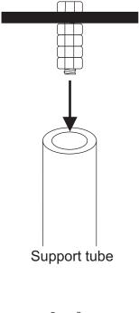
Insert this assembly into the support tube. Tension on the support ropes will hold it in place when the antenna is fully assembled.
