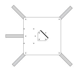
Install the support mast bracket using the longer  $6-32 \times 1-1/4$  screws supplied with the kit. The screws you removed will not be needed.
