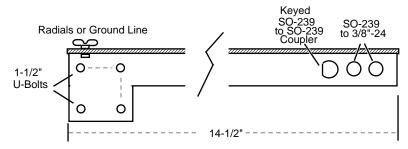
**Grounding Post:** A hole for mounting a ground-wire post is located above the U-bolt holes. This post may be used to connect radial wires, a counterpoise, or a earth safety ground. Install as shown below, using 10-24 hardware:
