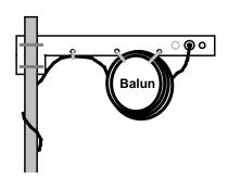
Lower HF Range: Coil 16-18 feet of cable Upper HF Range: Coil 6-8 feet of cable
