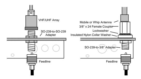
**Mounting Dipole Elements:** The dipole mount is configured differently because both legs of the antenna element must be electrically insulated from the arm. A portable dipole may consist of two hamsticks, two center or base loaded whips, a screwdriver paired with a fixed whip, or two MFJ heavy-duty collapsible stainless elements. Off-center feed may be used to facilitate matching. Element legs install using the two 1/2-inch holes located at the end of the mounting arm (see below):
