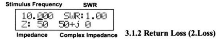
This function on the MFJ-213 reads the return loss and SWR of an antenna connected to the antenna connector. There are two modes in this function. The default is return loss and the next mode selected by pressing the **MODE** button is cable loss. The cable loss is measured by connecting the cable to the antenna connector and leaving the other end open or unterminated. This mode is for 50 ohm cables.
