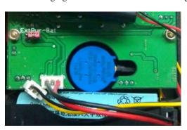
18650 battery will only charge when the MFJ-266B is off. For charging the position of the EXT PWR-BAT jumper does not matter. It will charge in either position.
