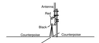
Counterpoise should lie on top of the ground. Do not anchor with a ground rod – it will de-tune the array. The center and far ends of the counterpoise wires may be secured with non-conductive stakes or pins to hold them in place.
