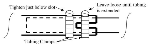
Figure 3: Tubing Clamp Positioning
