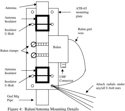
2) Attach radials to the ATB-65 using the 3/8" lugs under the U-bolt mounting hardware. Multiple radials can be attached to each 3/8" lug. Use as many radials as possible – preferably 16 or more - and make the radials as long as possible.
