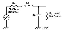
The solution for this type of network has three steps. First, calculate *network* Q, which is determined by the size (or magnitude) of the impedance transformation. The larger the impedance transformation ratio, the higher the Q requirement.
