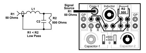
When configuring an N network of this type, note that the shunt capacitor (C2) is always installed at the high impedance end (R2). To facilitate this configuration, Capacitor-2 is wired in for the test. To find functional L/C values, use the same procedure you would for tuning with an antenna tuner. Step through the inductance settings and rotate the capacitor's tuning range at each stop. Find the value combination that delivers the lowest SWR.
