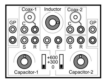
**1). GP Posts:** "General purpose" binding posts located on each side of the panel are disconnected from the internal tuning elements and may be used for supporting and connecting external (add-on) components.
