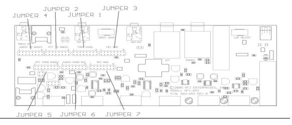
Figure 4: MFJ-652 Internal Jumper Blocks
