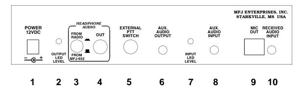
Figure 2: MFJ-652 Rear Panel Jacks and Controls
