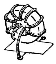
A turn is one complete "lap" around the toroid. The winding begins and ends with a halfturn to form its mounting leads. Therefore, it appears at first to have 9 turns. In fact, if you count 8 complete loops plus a short lead on each side for mounting, you have wound it correctly.
