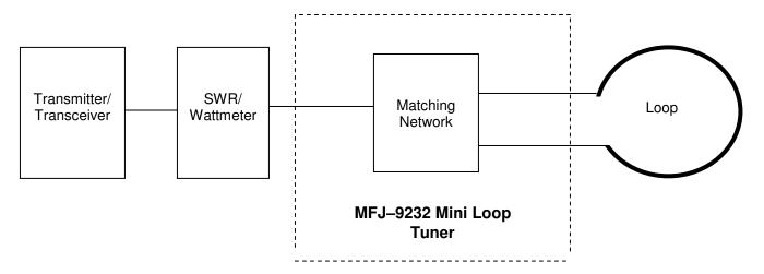
Figure 3: Typical MFJ-9232 *Mini Loop Tuner* <sup>™</sup> Configuration
