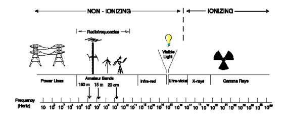
Figure 2: The Electromagnetic Spectrum
