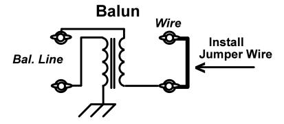
To place the balun in line and energize the *Bal. Line* terminals, connect a *Jumper* from the unbalanced *Wire* terminal post to the terminal post directly below it. The jumper-wire path is labeled on back panel for reference. Note that the *T-network* is always in line when the Antenna Selector is switched to the *Wire/Bal. Line* position.
