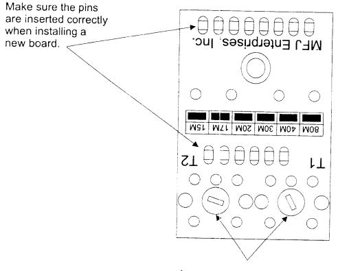
The board is oriented upside down as shown when installed into the radio.
