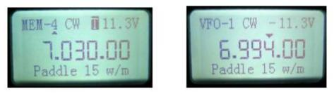
You can transmit on 40m band (7.0-7.3MHz). The screen display "T" when transmitting. The screen display "-" when you try to transmit outside band. No signal will be sent, but side tone works, you can use this as CW practice.
