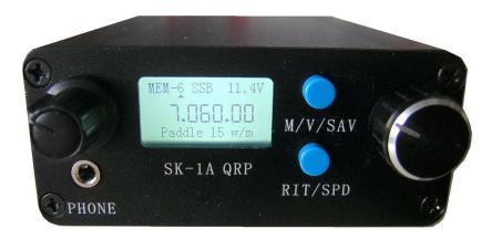
Specifications Size: 88\*38\*124mm (not including knob, etc.) Weight: about 280g (not including battery pack) Supply voltage: 10-15VDC Current drain Receive: about 60mA Transmit: about 800mA (DC12V) Receive: 5.9-8MHz Transmit: 7.0-7.3MHz VFO: DDS circuit with 50MHz reference frequency Display: LCD. Output power: 12V supply 5-6W,13.8V supply 8-9W Side tone: about 700Hz Automatic key: 5-40wpm adjustable Memory: 8
