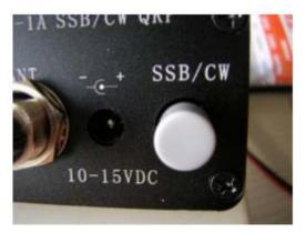
SSB/CW mode change switching is at back, push down is SSB, release is CW, screen shows the mode that you choose.
