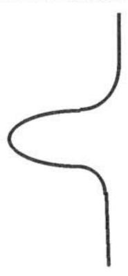
The wire insulation is removed where shown in the directions, and made into a half loop as shown above.
