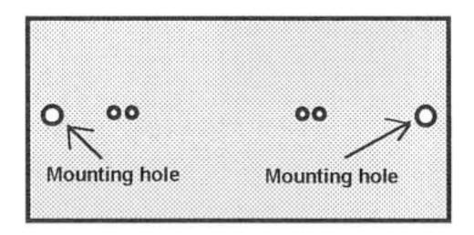
Now, make sure that the two screw pilot holes on the pine board for mounting the coil form are correct. Refer to the drawings in the manual that show the placement for the Fahnstock clips and coil form. Temporarily mount the coil in its proper location using two Phillips head screws. You do not need to fully tighten the screws, we are just checking to see that things fit properly.
