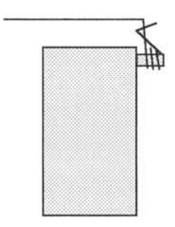
☐ Using the long nose pliers, gently twist the half loop to take up wire slack and tighten the wire wraps made over the stud.
