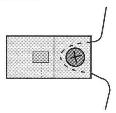
The above drawing shows a through connection being made to a Fahnstock clip. The dotted line shows where the wire runs under the clip body.
