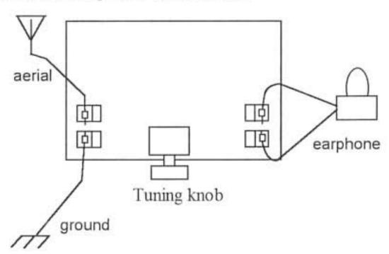
Connect the earphone wires to the Fahnstock clips at the right hand side of the radio.
