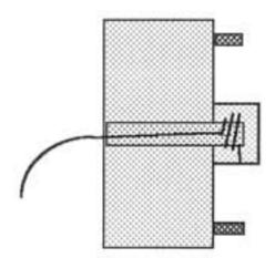
☐ Gently, but firmly, squeeze the turns wrapped around the rotor lug, using the long nose pliers, until they are compressed tightly--making a good, tight electrical connection.
