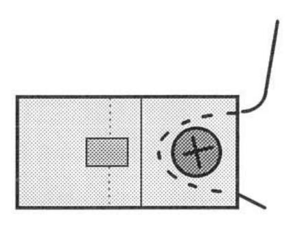
Through connections are used when the wire goes to a electrical connection at a Fahnstock clip, and then continues on to make one or more connections to other points. The directions will tell where to make a through connection on a wire, and how much insulation needs to be removed.
