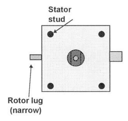
This is the correct orientation for installing the capacitor. Note that the narrower rotor lug must be at the left hand side!
