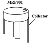
□□ 2. Locate the silk-screened footprint for Q1, almost dead-center on the PC board. Note that the long collector lead is oriented toward
