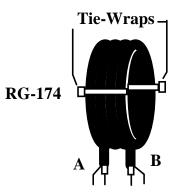
4. Install the ends of the RGS-316 at T1, as shown in the following diagram, and solder in place. Note that the coax shield on the L1 side of the balun (A) should be connected as shown (to the foil or grounded side of the PC board).
