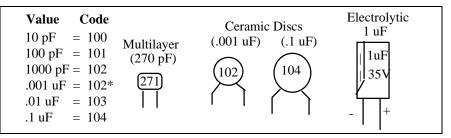
As with resistors, it's helpful to sort capacitors by type, and then to arrange them in ascending order of value. Small-value capacitors are characterized in pF (or pico-Farads), while larger values are labeled in uF (or micro-Farads). The transition from pF to uF occurs at 1000 pF (or .001 uF)\*. Today, most monolithic and disc-ceramic capacitors are marked with a three-number code. The first two digits indicate a numerical value, while the last digit indicates a multiplier (same as resistors).
