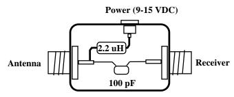
Warning--do not reverse direction when installing
