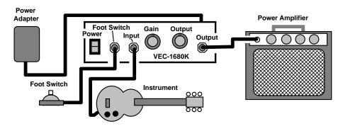
**Foot Switch:** To bring the preamp on-line, simply close the foot switch. The internal relay re-routes the audio path through the preamp circuitry. To bypass the preamp, open the foot switch.
