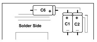
Flip the PC board over to its *solder side* and mount the 10 uF caps as shown:
