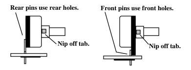
□ □ On the *solder side* of the PC board, mount a 500K pot at R9 and solder.
