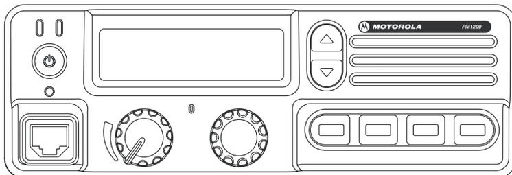
PM1200 is a full featured FM transceiver, designed for flexible mobile and base station business communications in the VHF Low-Band frequency range (120/50 Watts: programmable). Each model is designed for reliable business communications in a wide variety of applications, with a wide range of operating capability provided by its leading-edge design.
