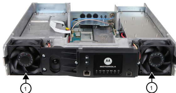
Figure 4: Front view (without top and bottom covers) of the SLR 8000 Base Station/Repeater
