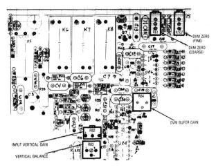
Figure 5-14. Front Panel Interface Alignment Points
