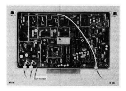
Figure 10-3. Receiver Parts Locator
