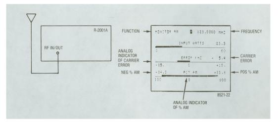
Figure 4-4. System Analyzer Time Base Calibrate Test Setup and CRT Display
