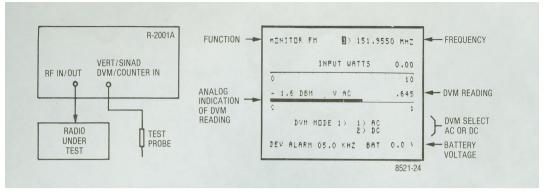
Figure 4-10. Test Setup for Using DVM and Signal Generate with CRT Display
