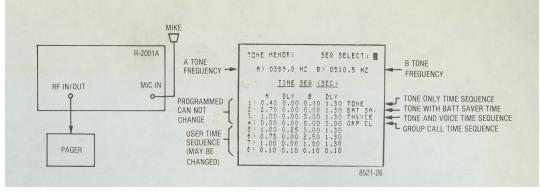
Figure 4-9. Test Setup for Pager and Alert Functions with CRT Display
