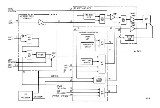
Figure 5-11. Oscilloscope Block Diagram
