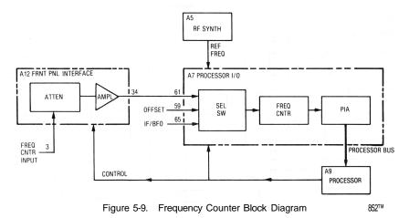
5-67. The external input signal is routed to the Front Panel Interface module (A12). A range Attenuator on the Interface module provides variable sensitivity settings according to the vertical range switch setting on the front panel. An Amplifier following the range Attenuator amplifies and limits the signal amplitude for the frequency counter input.
