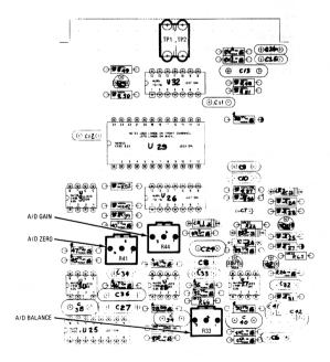
Figure 5-19. Processor I/O A/D Alignment Points
