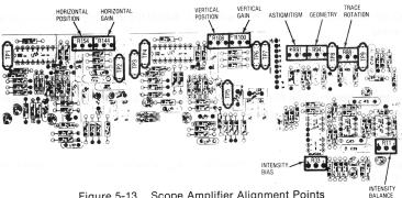
Figure 5-13. Scope Amplifier Alignment Points
