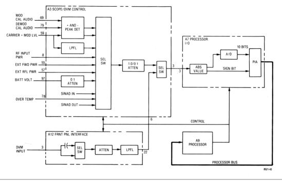
Figure 5-10. Digital Voltmeter (DVM) Block Diagram
