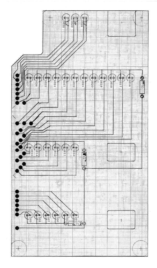
Figure 20-2. Display Board A14A1 Schematic Diagram (01-80304A43)
