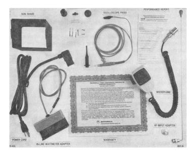
Figure 2-1. Accessories Supplied with Analyzer
