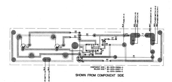
RTP-1002A Battery Pack Schematic Diagram, Circuit Board Detail, Parts Location Detail, and Parts List Motorola No. PEPS-29554-O (Sheet 1 of 2) 3/24/80-SK
