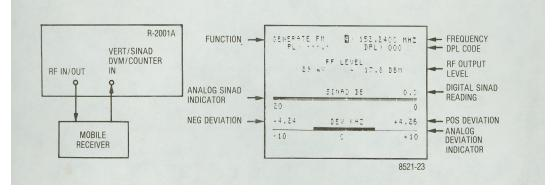
Figure 4-8. Test Setup for FM Receiver Sensitivity Using Generator and SINAD Meter with CRT Display
