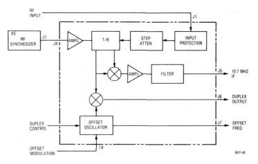
Figure 5-7. Duplex Generator Block Diagram
