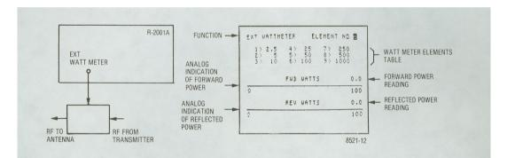
Figure 4-7. Wattmeter Test Setup and CRT Display
