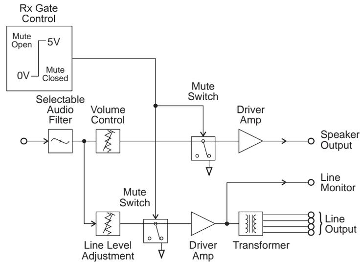
**Figure 2.3** T855 Audio Processor Block Diagram
