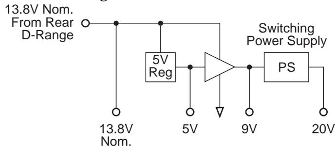
*Figure 2.4 T855 Power Supply And Regulator Block Diagram*
