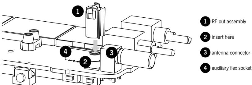
Figure D-12: Assembly of the switches (Orca Elan and Orca Excel)
