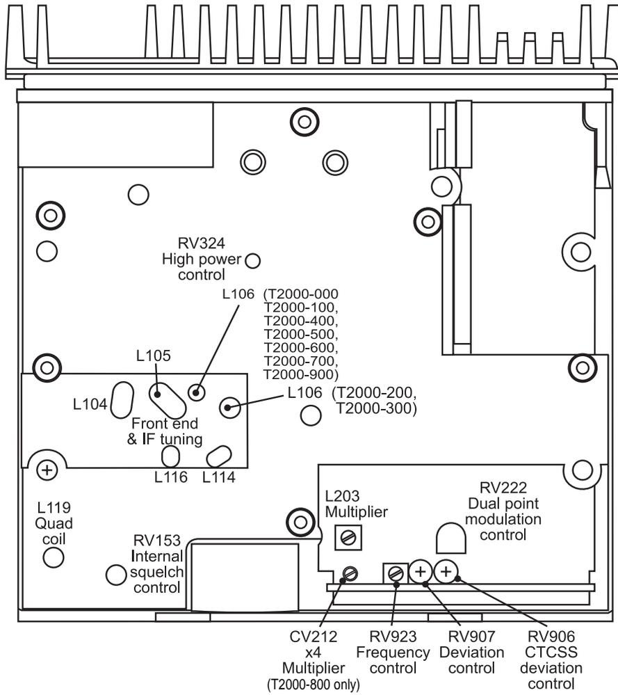
Figure 6.1 RF & TXCO/Tx Audio PCBs - Tuning & Adjustment Points-
