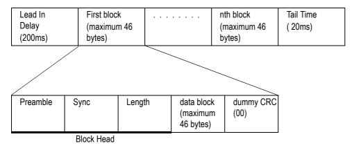
The default Transparent mode Lead In Delay is set to 200 ms. If a faster data rate is required the Lead In Delay can be reprogrammed to a minimum of 40 ms using the PROGRAM command. Note that if the Lead In Delay is set this low, Economy mode **must** be disabled.
