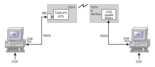
The A75 is fitted to a T201X radio and is connected to a personal computer (PC) by a serial line using five standard RS232 signals (TXD, RXD, CTS, RTS and GND).
