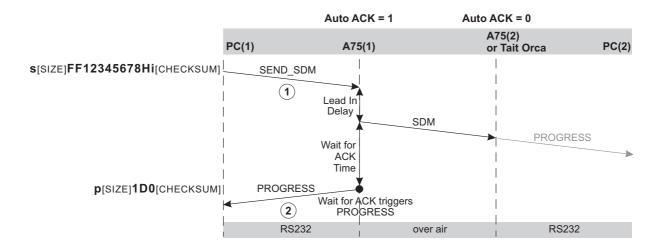
SDM Auto ACK is either enabled or disabled when the modem is configured. This is done in the A75 with the PROGRAM command or in the PGM programming software for the Tait Orca. If the A75 has SDM Auto ACK is set to '1' (enabled) in bit 7 of the [ITEM1] parameter of the PROGRAM command, then:
