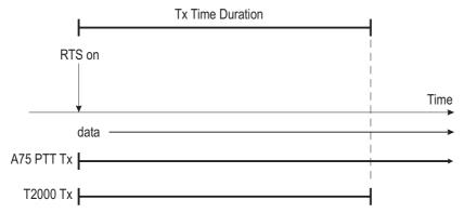
If the radio transmitter times-out in this way, it can not transmit data again unless RTS is turned off then on again.
