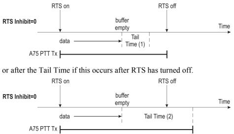
If the data stream has a gap, while RTS remains on, the A75 continues to transmit. This eliminates the data delay caused by the Lead In Delay at the start of each transmission.
