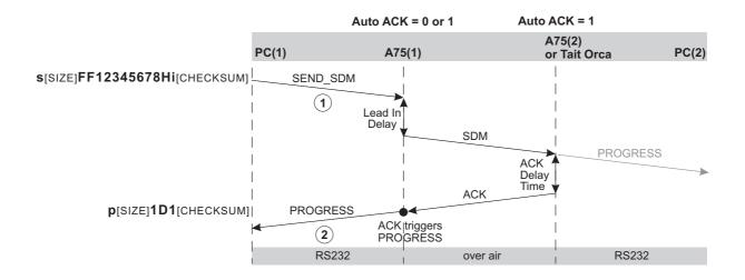
In the example above, the receiving modem A75(2) has the SDM Auto ACK enabled so an 'ACK' is returned to the A75(1). When the A75(1) receives the 'ACK', it generates a **PROGRESS** message (2), of [PTYPE] SMD ACK (1D) with the flag set to '1' (ACK Received). Refer to the PROGRESS command details for further information.
