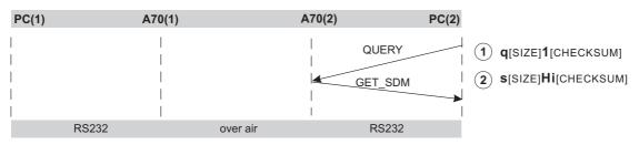
When it receives the SDM QUERY command, the A75 responds with a GET\_SDM message (2). If there is no data in the EEPROM then the GET\_SDM is returned with an empty [PA-RAMETERS] field.
