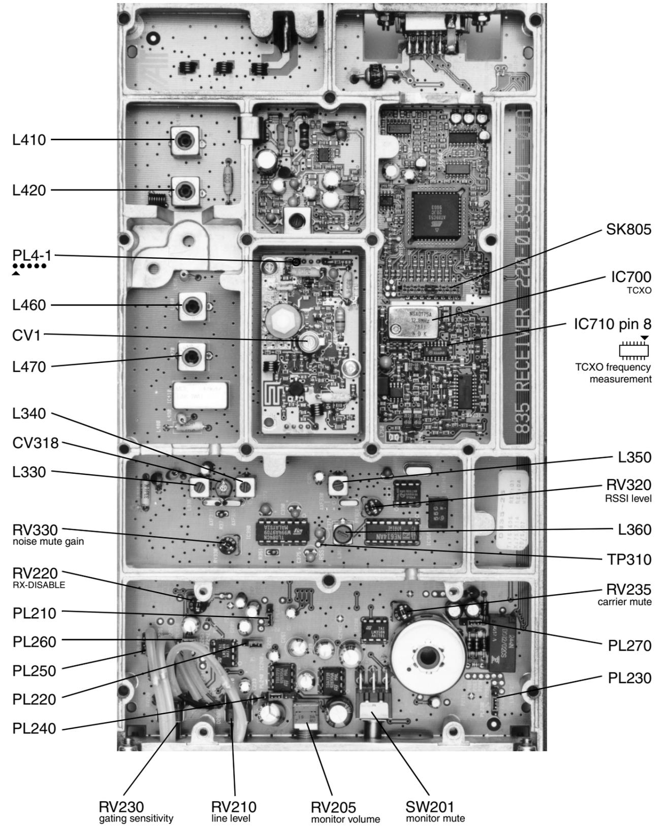
The photograph printed at right will help you to identify the main controls used in tuning and adjusting the T835.
