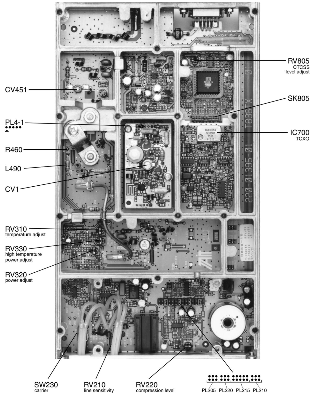
Figure 4.4 T836 Main Tuning & Adjustment Controls
