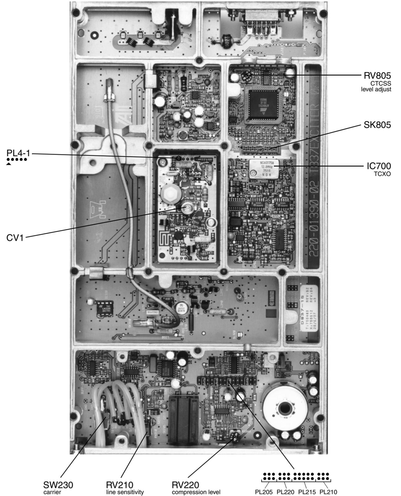
The photograph printed at right will help you to identify the main controls used in tuning and adjusting the T837.
