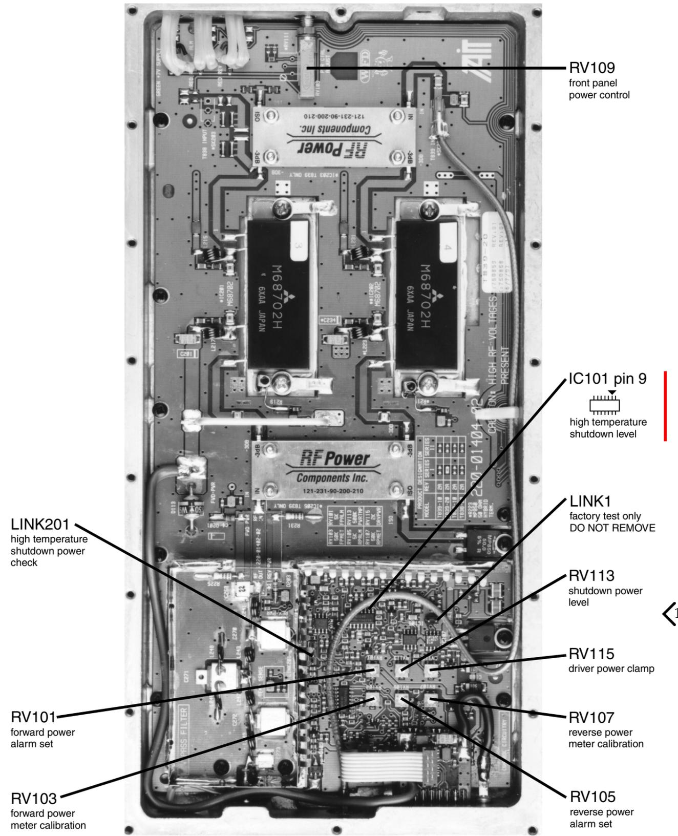
Figure 3.3 T838/839 Main Adjustment Controls (T839 Shown)
