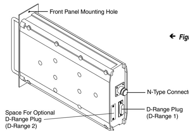
← Figure 1.2 T835 Chassis Connectors
