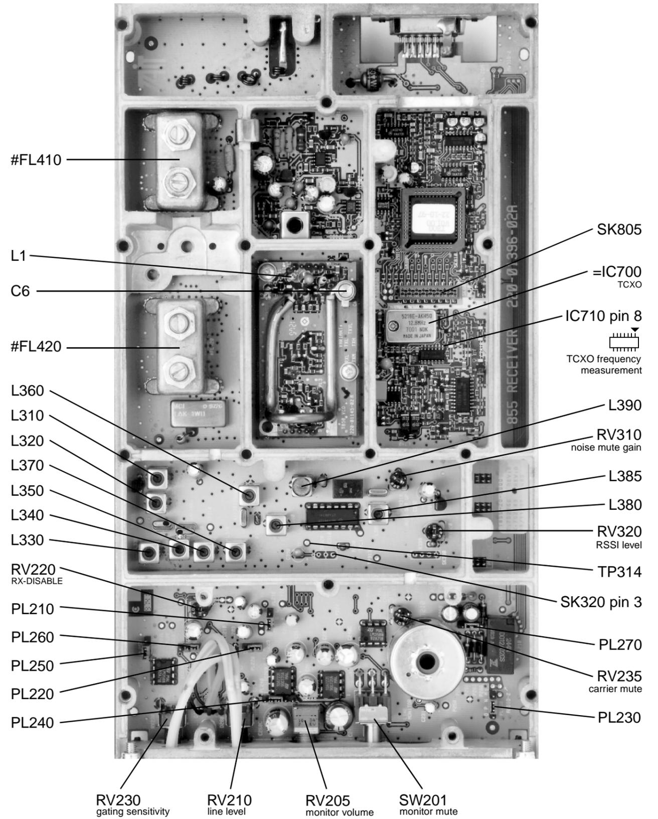
The photograph printed at right will help you to identify the main controls used in tuning and adjusting the T855.
