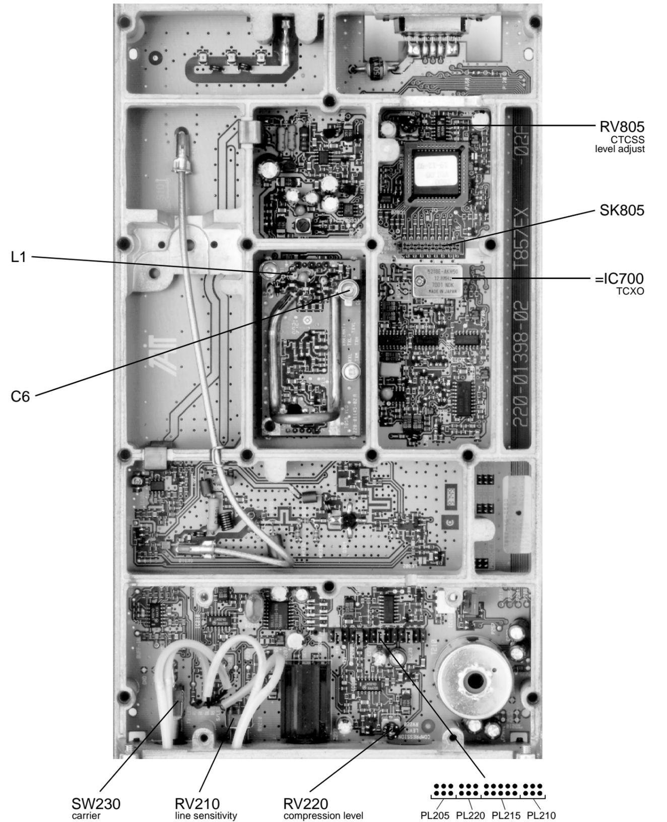
The photograph printed at right will help you to identify the main controls used in tuning and adjusting the T857.
