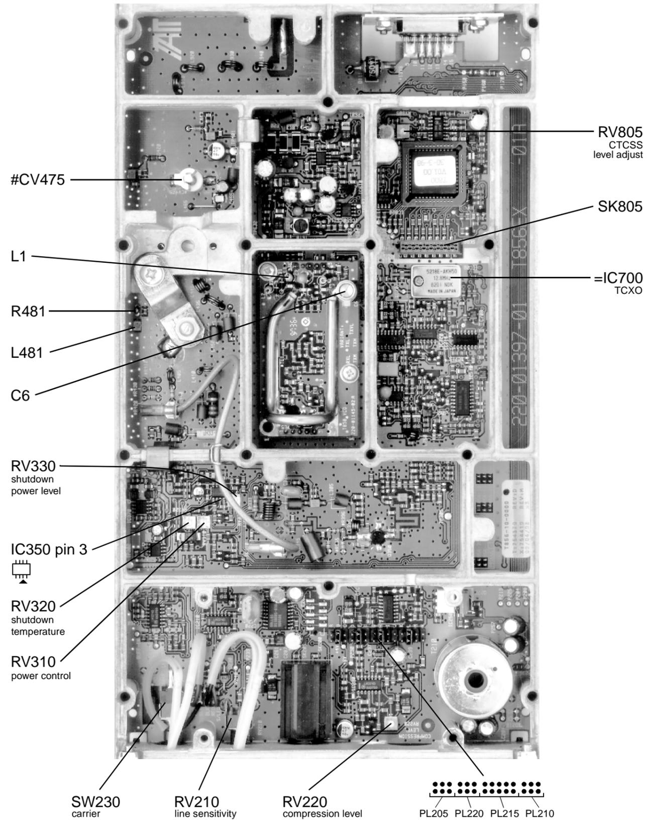
Figure 4.4 T856 Main Tuning & Adjustment Controls
