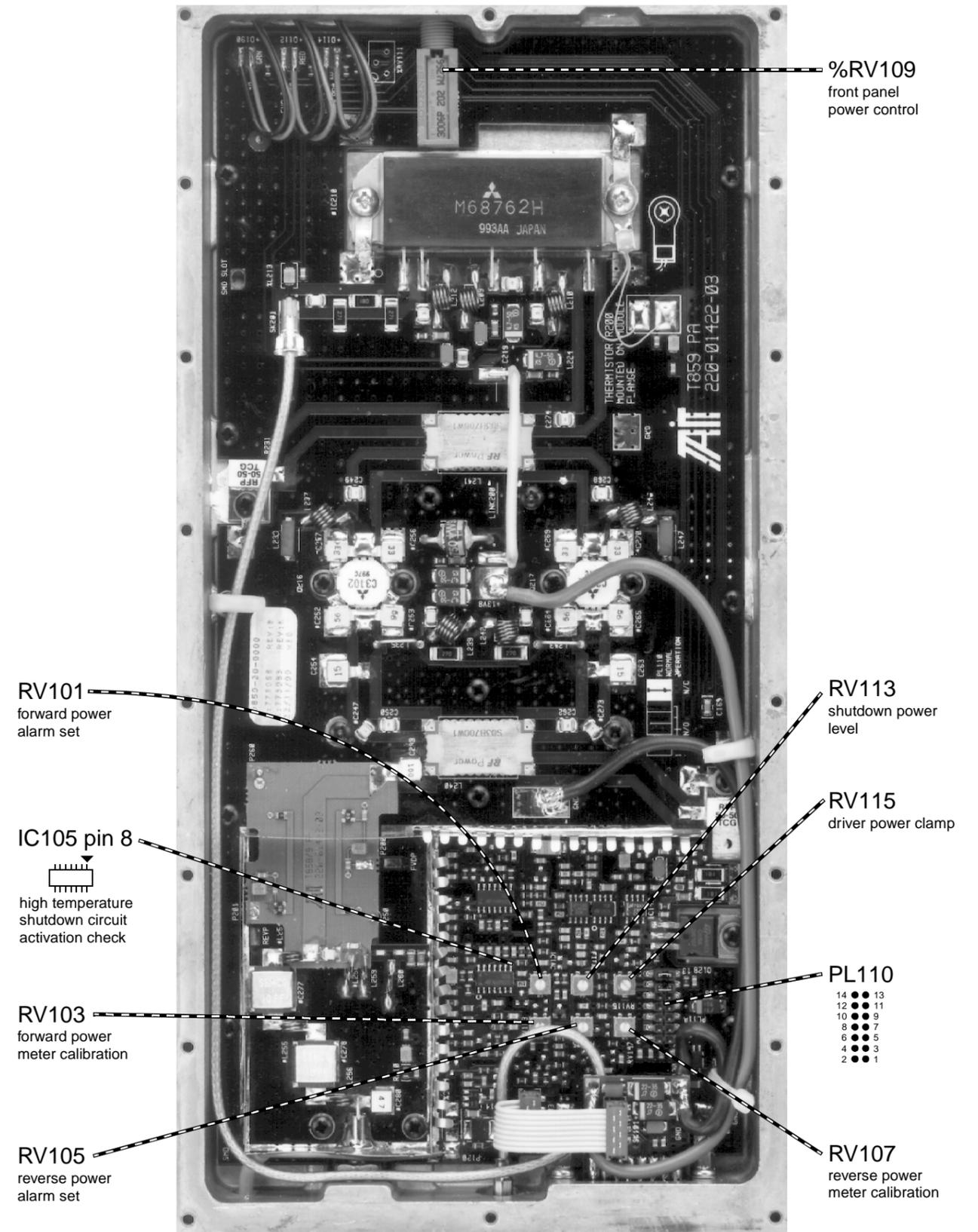
The photograph printed at right will help you to identify the main controls used in adjusting the T859 with RF power module.
