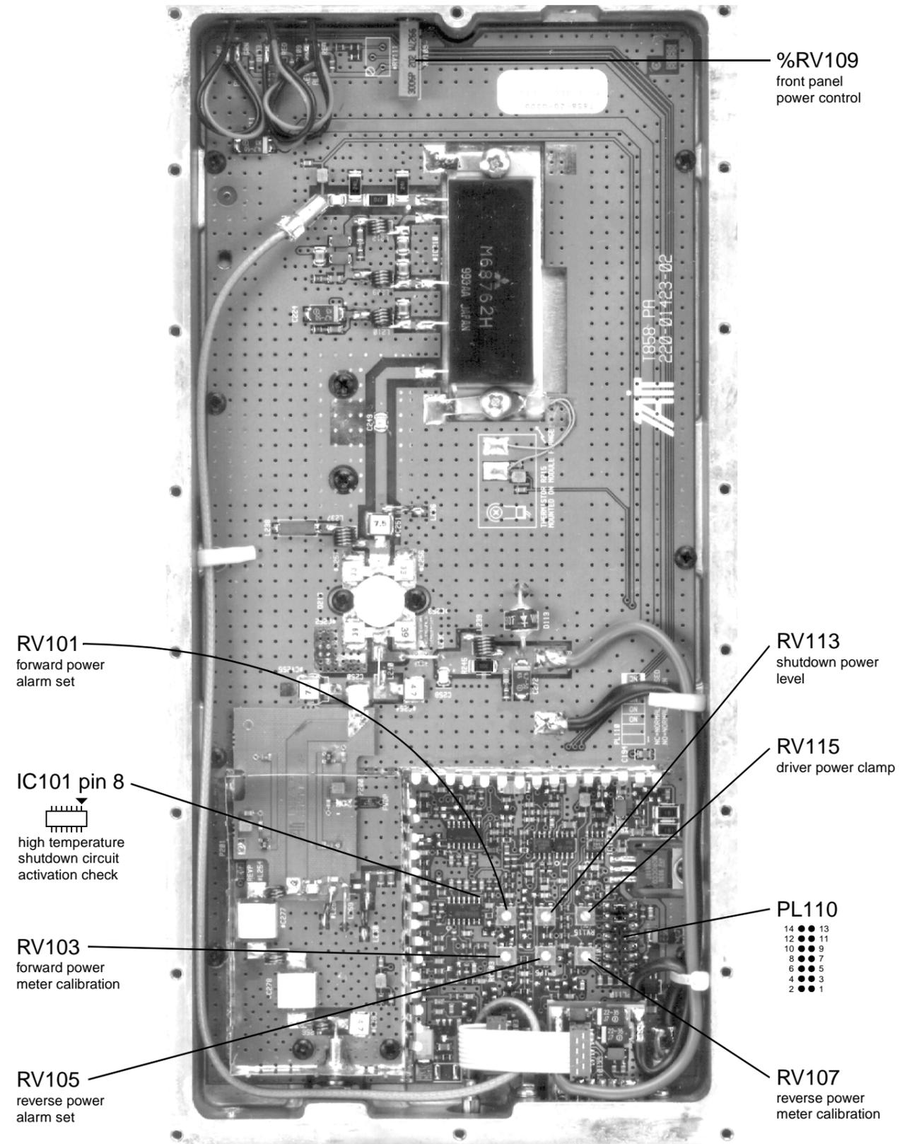
The photograph printed at right will help you to identify the main controls used in adjusting the T858 with RF power module.
