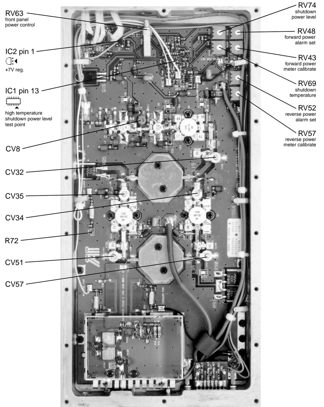
The photograph printed at right will help you to identify the main controls used in tuning and adjusting the T858 without RF power module.
