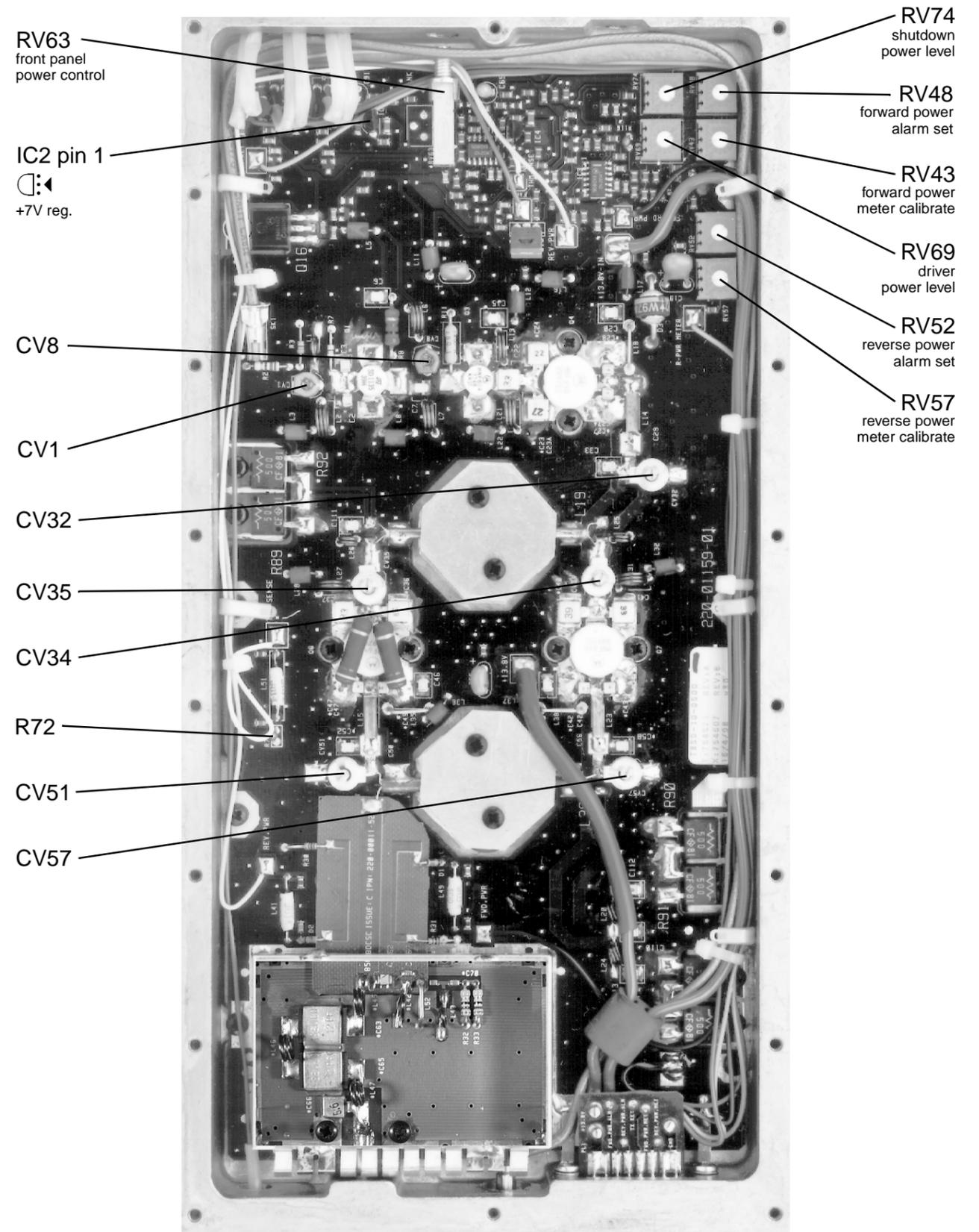
The photograph printed at right will help you to identify the main controls used in tuning and adjusting the T859 without RF power module.
