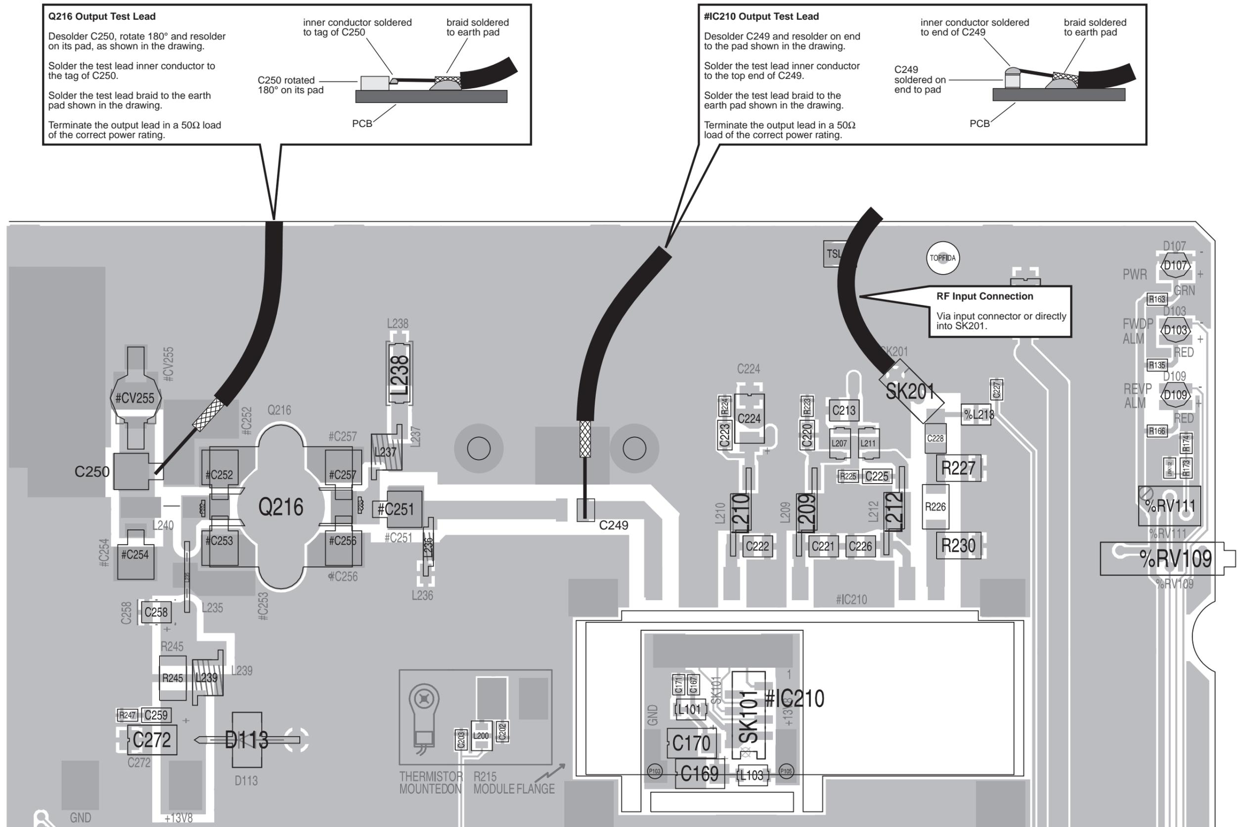
Figure 4.3 T858 Test Break Point Location
