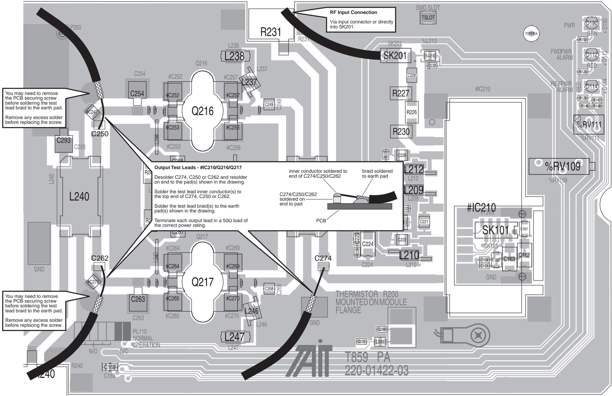
Figure 4.4 T859 Test Break Point Location
